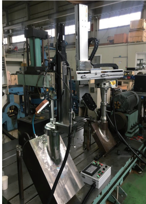
Figure 8. UNSM equipment on CRDM nozzle mockup.
