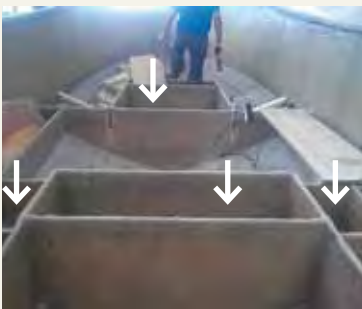
Manufacturing of helium tanks using bulkheads
