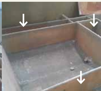
Manufacturing of helium tanks using bulkheads
