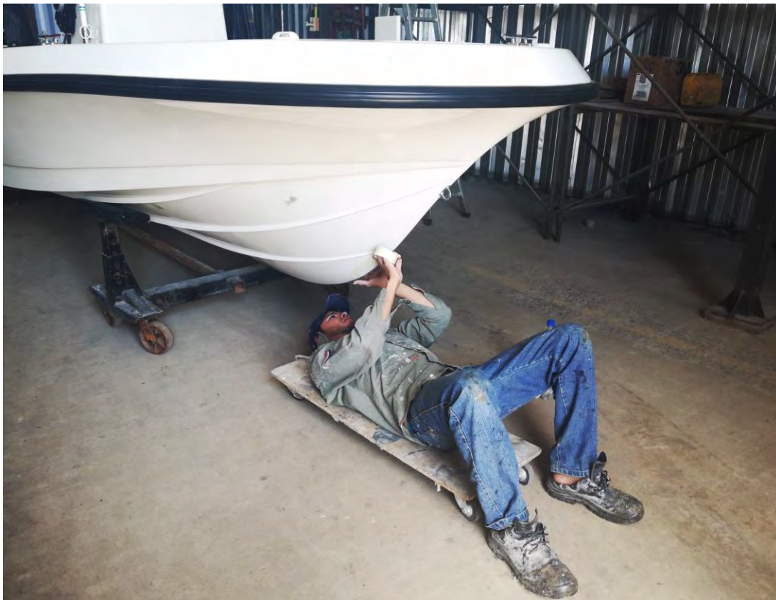
Oscar patching some gel coat damage.
